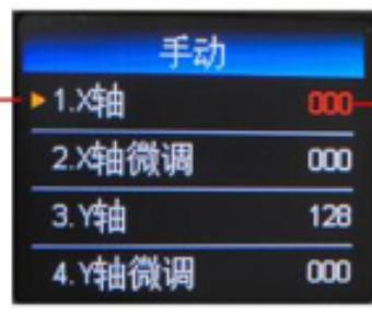
(2) Press "OK" key enter into Edit status, the word is red, then press "UP" "DOWN" to select, press "OK" save and Exit edit status.
