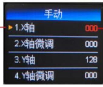
(2) Press "OK" key enter into Edit status, the word is red, then press "UP" "DOWN" to select, press "OK" save and Exit edit status.
